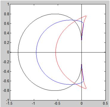
ldtab3 =(E\*du)./(E\*ab3); plot (ldtab3 ,'r-'); % AB3 bdf3ex3=(E\*bdf3)./(E\*ex3); plot (bdf3ex3,'b-'); % BDF3/EXT3 bdf2ex2=(E\*bdf2)./(E\*ex2); plot (bdf2ex2,'k-'); % BDF2/EXT2 -
