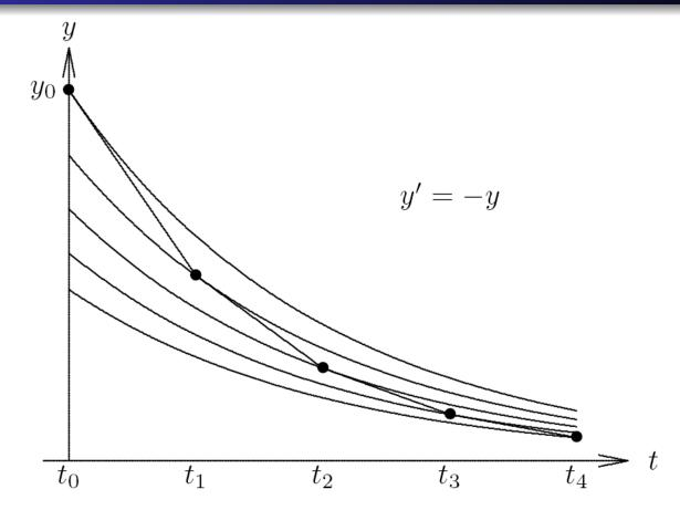
For stable solutions, errors in numerical solution may diminish with time (Local errors are suppressed.)
