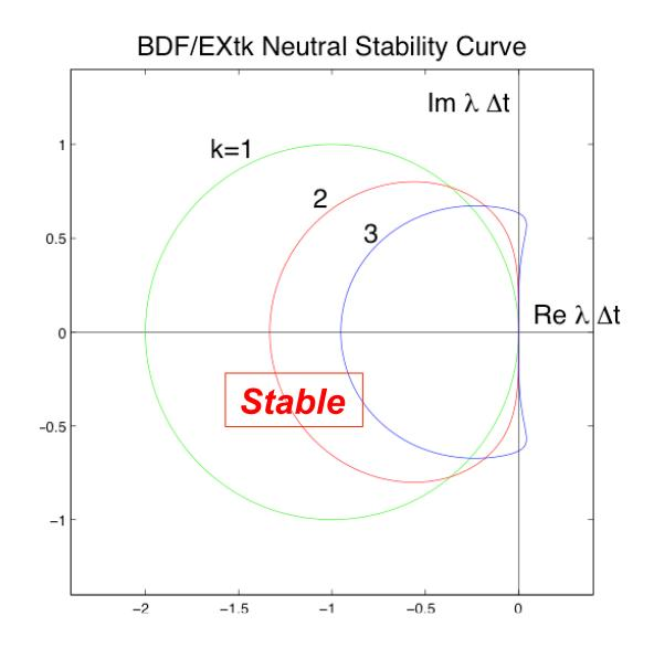
□ Here we see that the k=3 curve encompasses part of the imaginary axis near the origin of the  $\lambda \Delta t$  plane, which is important for stability of non-dissipative systems.
