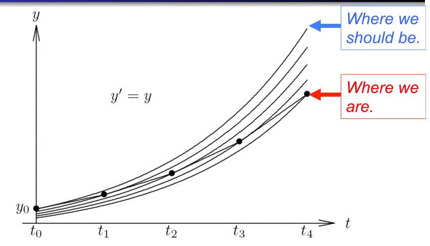
For unstable solutions, errors in numerical solution grow with time
