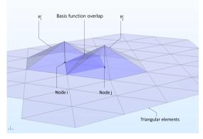
We partition the domain into triangles (elements) and define linear basis functions that are 1 at the intersection of three or more elements (nodes).
